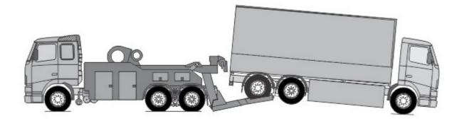
In case of a physical damage or a thermal event on the lithium-ion batteries, it is recommended to tow an electric truck with the rear wheels lifted.
