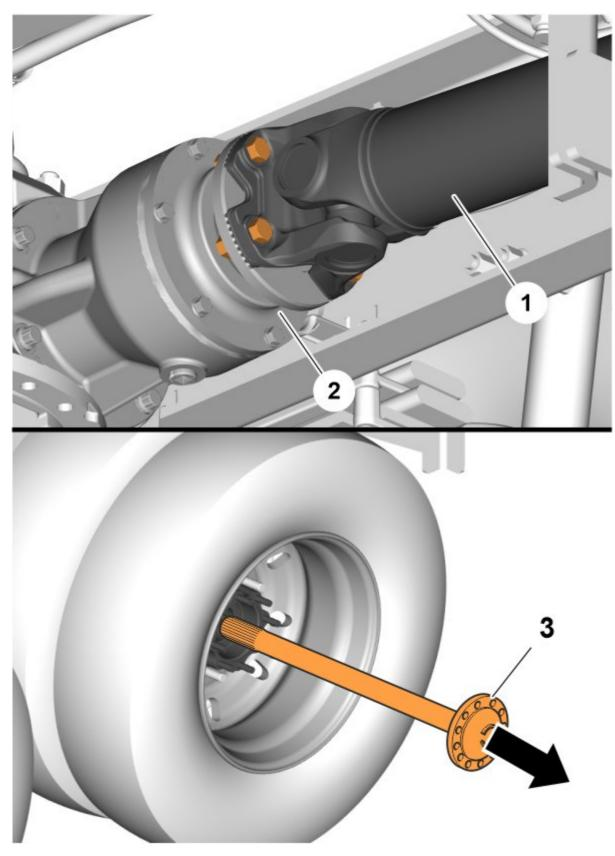
The drive to the rear wheels is disabled by either uncoupling the propeller shaft (1) from the driven axle (2) or by removing the axle shafts (3).
