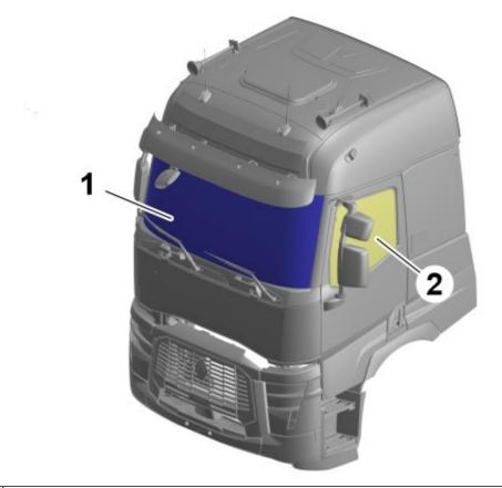
• The windscreen is made of laminated glass (1). The window glasses are made of tempered glass (2).
