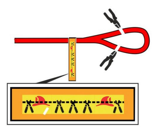
• Cut the emergency cut-off loop on each side of the loop to disconnect the traction voltage supply from the traction batteries.
