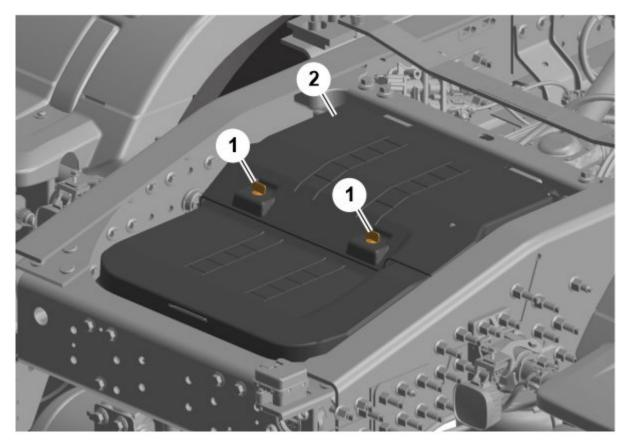
The 12 V batteries are located at the rear end of the truck.
