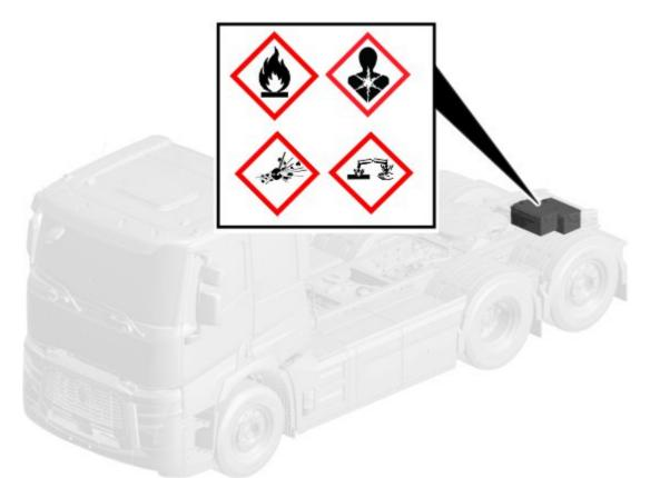
The electrolyte solution in 12 V batteries contains sulphuric acid, which is highly corrosive and can cause severe chemical burns to the skin and damage the eyes. The solution is also poisonous if ingested.
