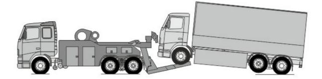
If the vehicle is towed with the rear wheels on the ground, it is mandatory to disconnect the drive to the wheels.
