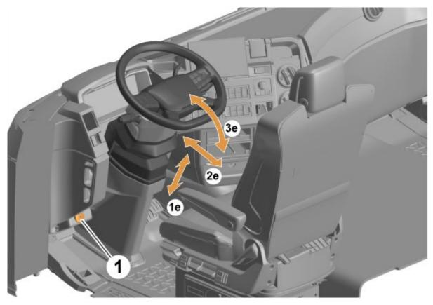
Press the control (1) to the position to adjust the steering column in the vertical (1e), lateral (2e) and angular directions (3e).
