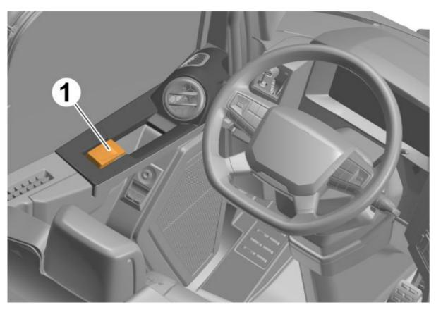
To open the door from inside the cab, lift the handle (1) and push the door.
