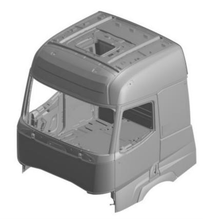
• The cab has no high-strength or ultra-high-strength steel. The cab structure is made of plain carbon sheet steel that will not exceed the yield strength of 420 MPa.
