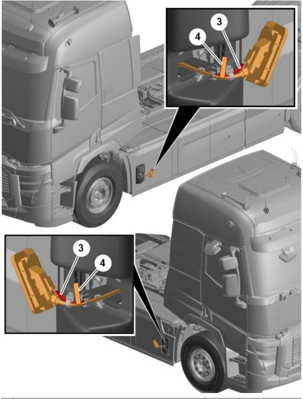
Pull out the marker lamp cable and locate the emergency cut-off loop (low-voltage) (3) with the label (4).
