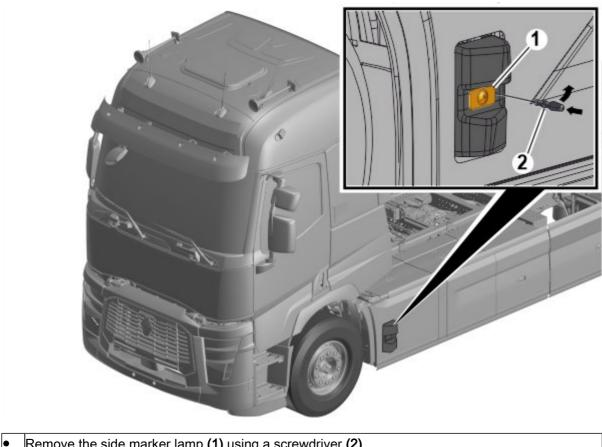
Remove the side marker lamp (1) using a screwdriver (2).
