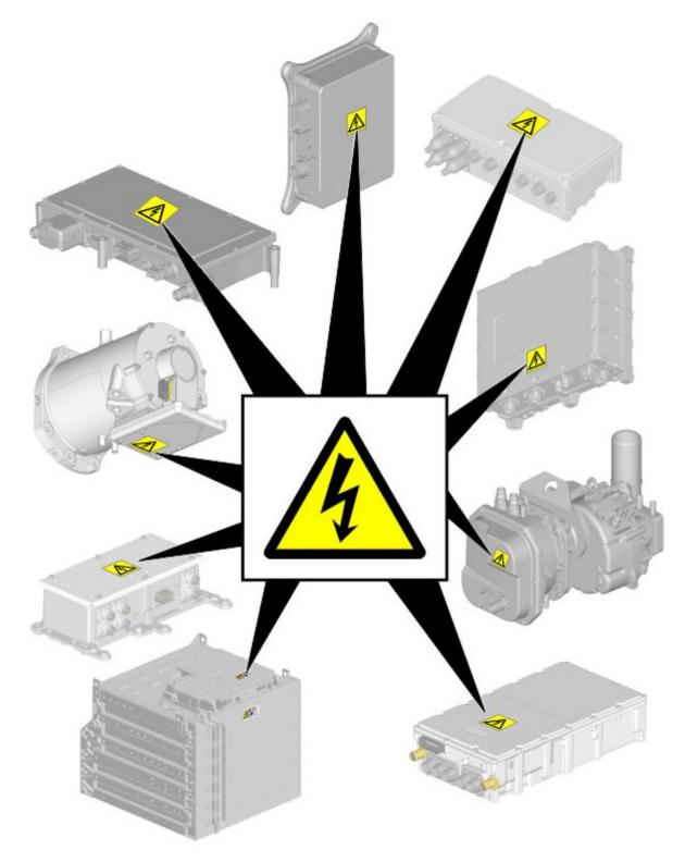
Most of the traction voltage components are marked with the warning label for hazardous voltage.
