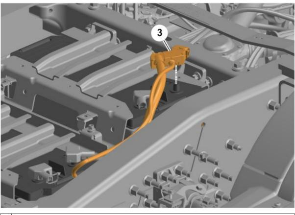
• Remove the battery negative terminal (3).
