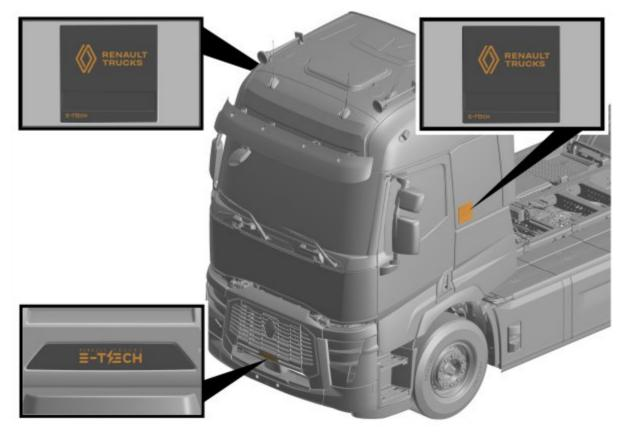
A BEV (Battery-Electric Vehicle) is identified by the 'E-TECH' emblem located on the front of the cab and near to the cab doors on both sides.
