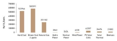
Use phase emissions from production of electricity. In the graph selected electricity sources are presented
