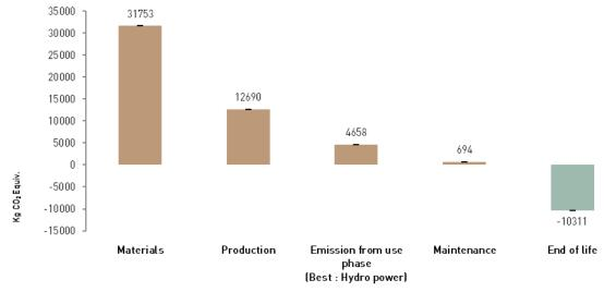
Global warming potential for the different life cycles of Renault Trucks D Wide Z.E.. The use phase shows the best case.
