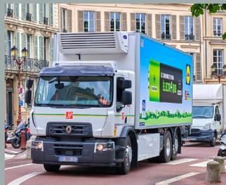
The Renault Trucks E-Tech D and D Wide models of 16 and 26 tonnes, which are produced in series, have been joined by an E-Tech D Wide adapted to temperature-controlled distribution missions.
