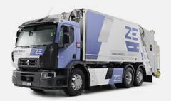
5 battery configurations, up to 6 battery packs of 66 kWh for a range of up to 400 km.
